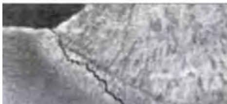
Welding Inspection: Crack through HAZ
