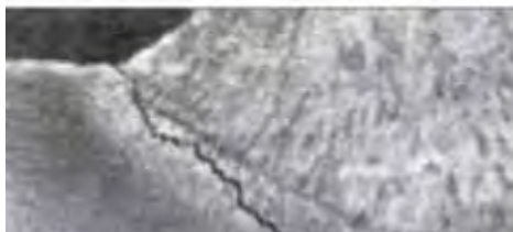
Welding Inspection: Crack through HAZ
